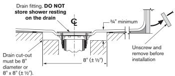
If opening is larger it must be adjusted to 8" x 8" with structural material (such as wood, cement, etc.) to prevent flexing.
